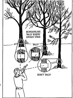
Figure 2....Point Sampling With An Angle Gauge
